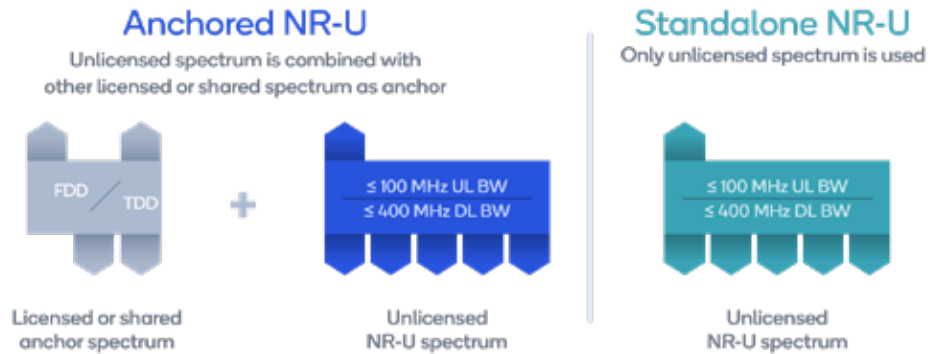
Fig.6 – NR-U Can be deployed in Anchored or Stand Alone mode
